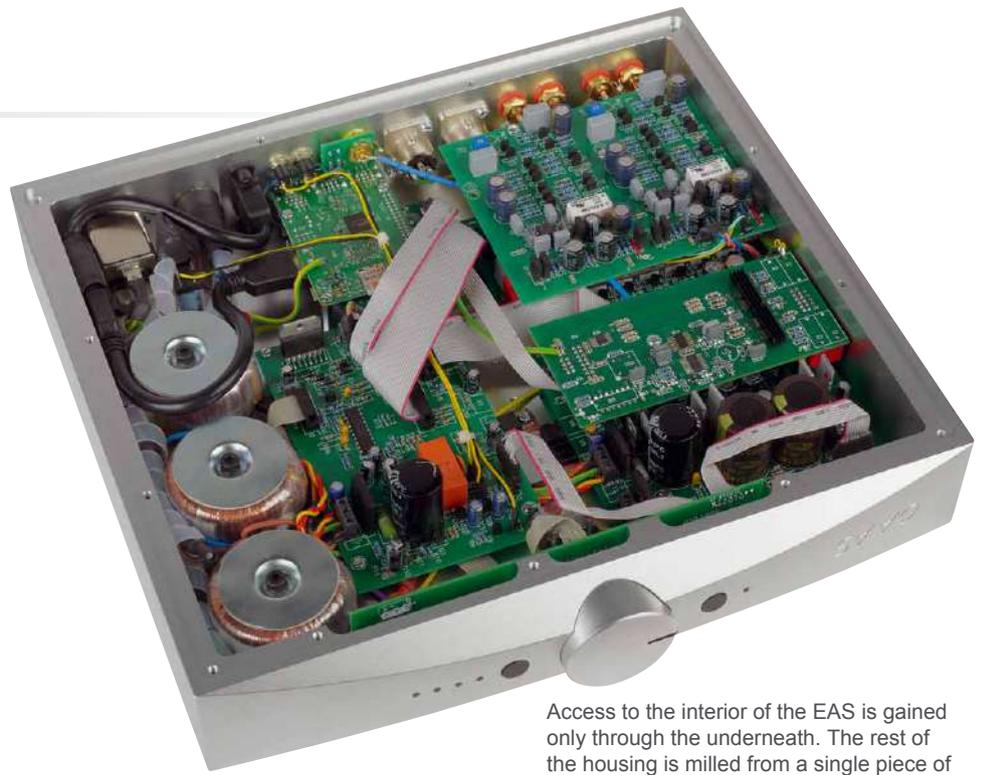
Access to the interior of the EAS is gained only through the underneath. The rest of the housing is milled from a single piece of metal
