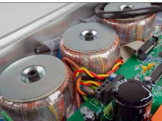
Three transformers mounted in the EAS, provide power to each one of the boards, Streamer, DAC and pre-amplifier
