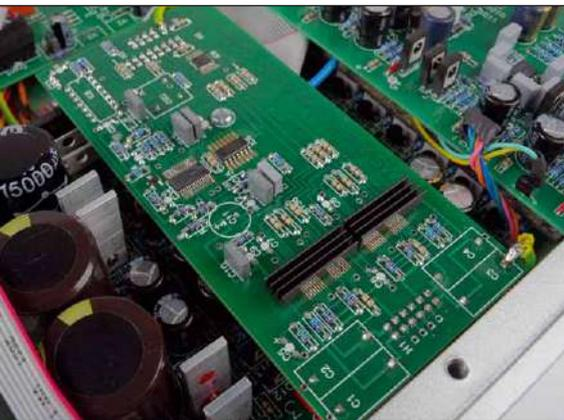
Digital data from the streamer is routed via I<sup>2</sup>S to the separately operating DAC Board. The two parallel DAC chips deliver great sound
