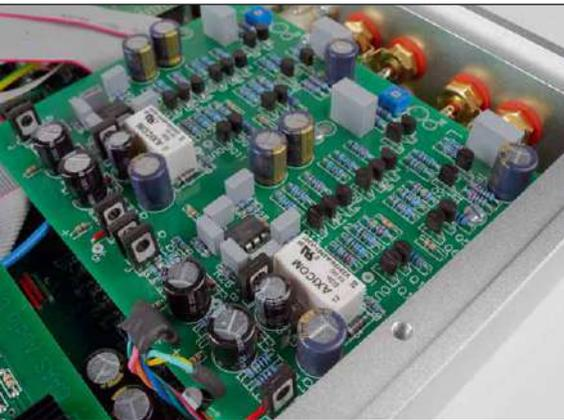
A true Class-A amplifier module is used in the pre-amplifier stage, which can adjust the volume in 128 individual steps
